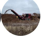
Finished compost is screened, removing large particles, and mixed into a soil amendment for sale.
